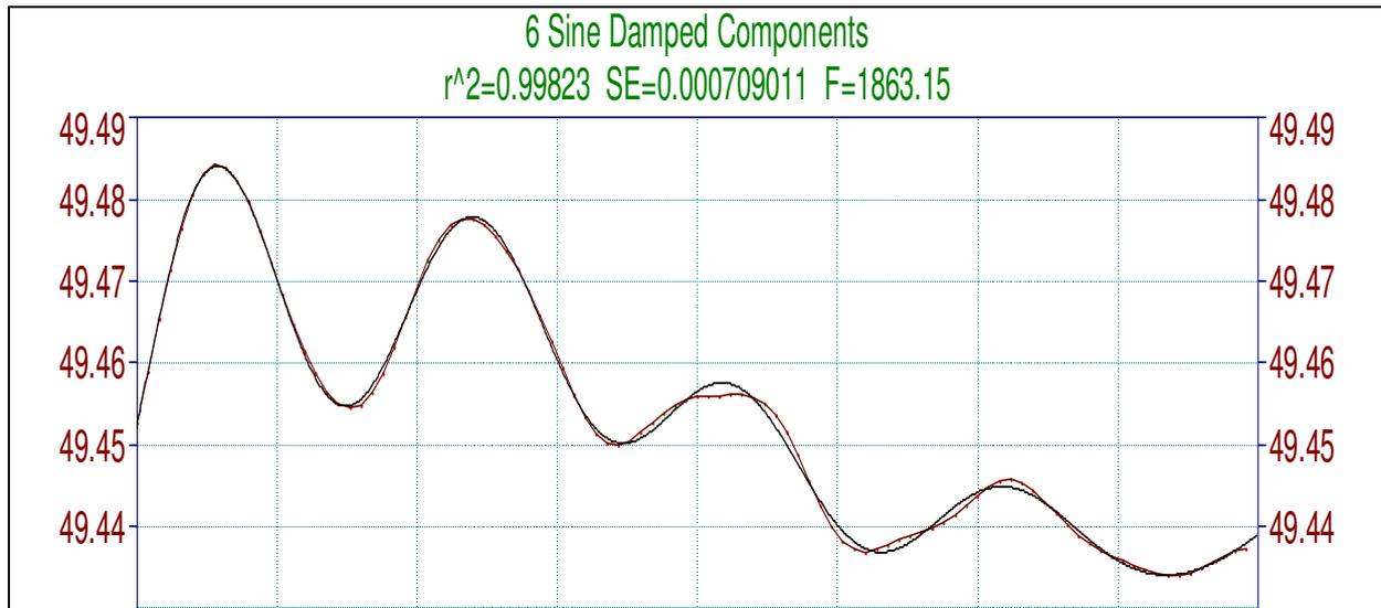
Figure 128: Prony Analysis of Frequency using 6 exponentially sine damped case
