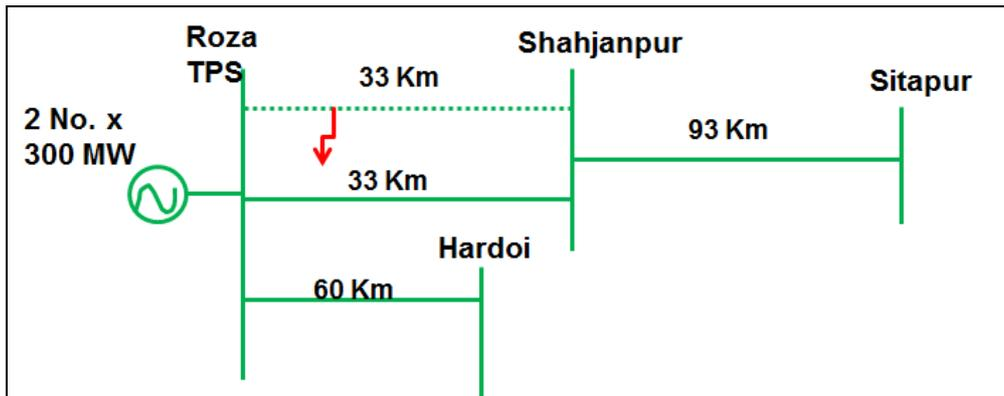
Figure 61: Connectivity diagram of Roza TPS in Northern region
