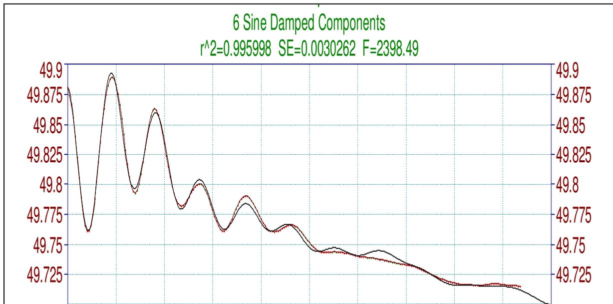
Figure 127: Prony Analysis of Frequency using 6 exponentially sine damped case
