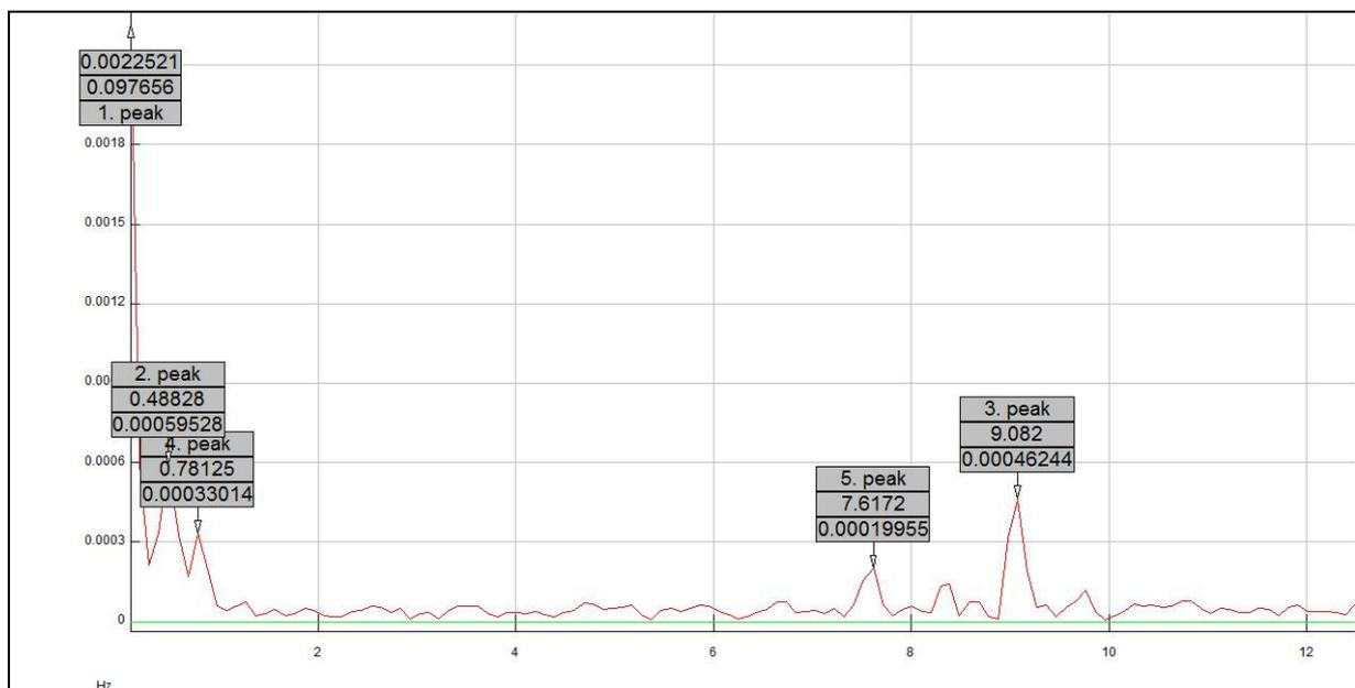
Figure 116: FFT of frequency at Raipur (HVDC B'wati flow is 750MW)
