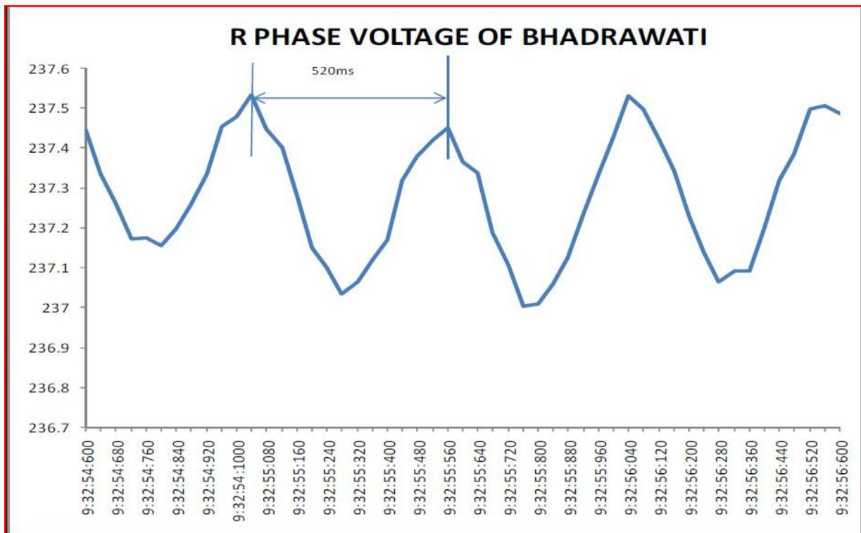
Figure 113: R phase voltage at Bhadrawati showing frequency of oscillations
