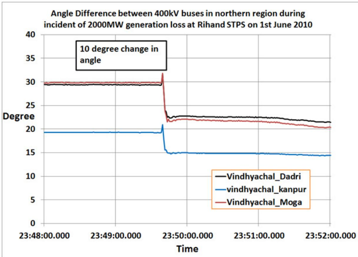
Figure 47: Angular separation during generation loss at Rihand
