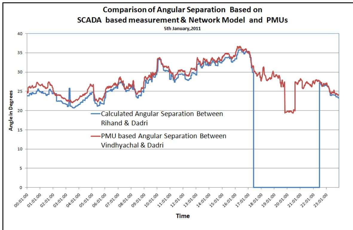
Figure 84: Comparison of Angular Separation based on SCADA measurement and PMUs
