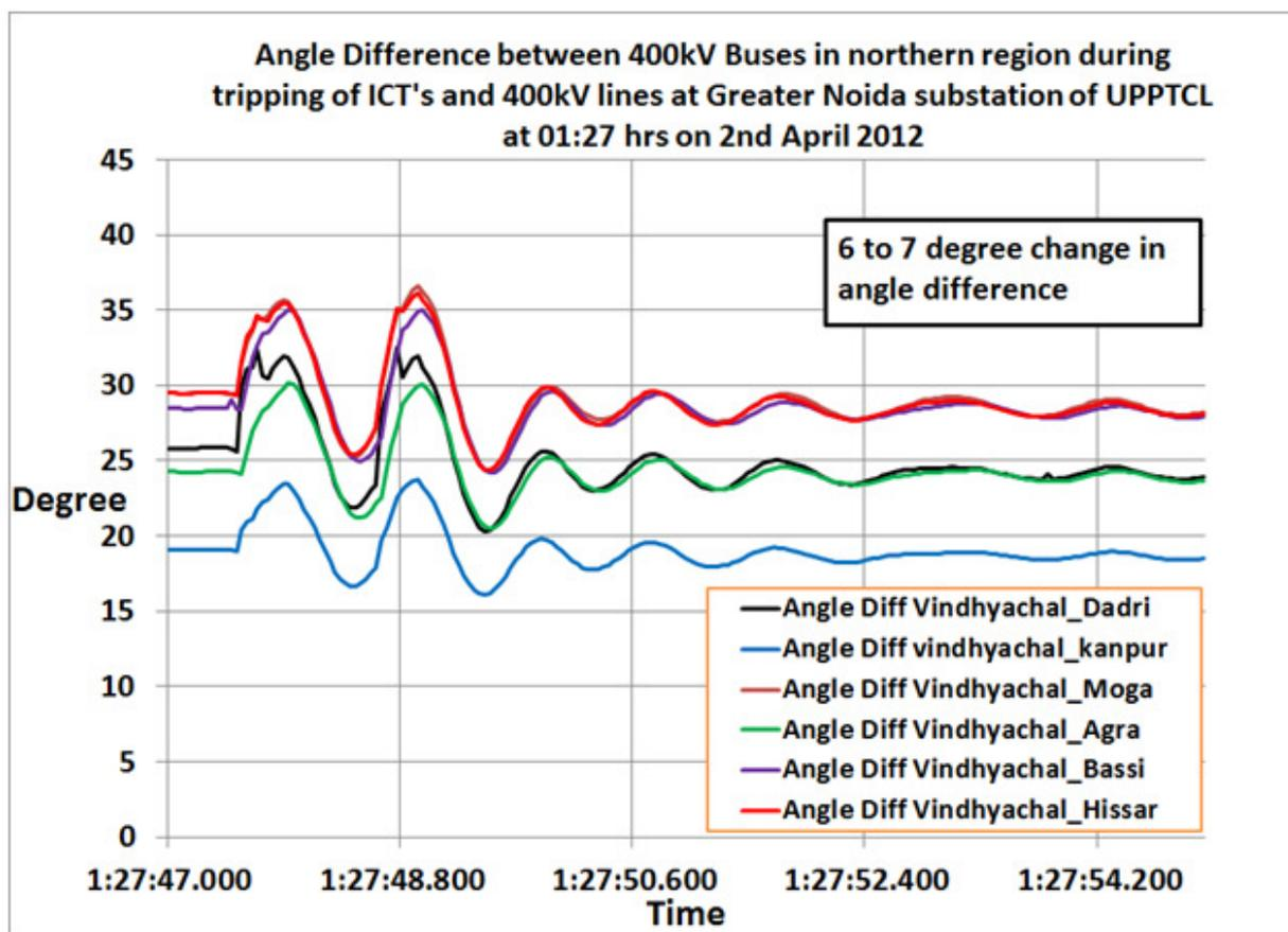
Figure 46: Swing observed in angles during multiple trippings at 400 kV Greater Noida
