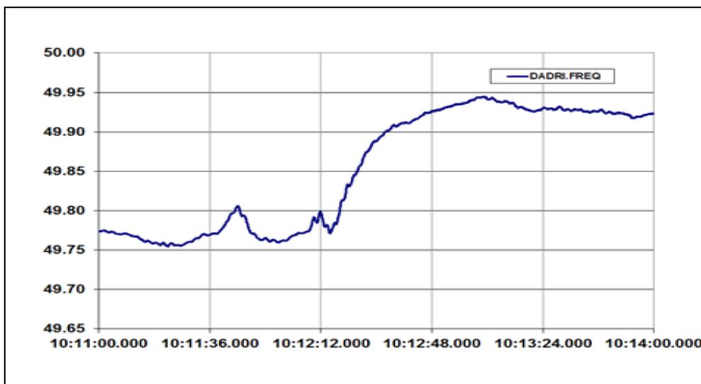
Figure 60: Increase in frequency during the incident in Punjab due to loss of load
