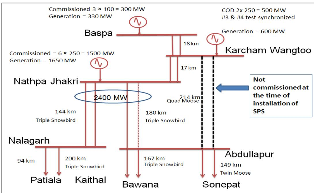
Figure 90: Connectivity diagram of Nathpa Jhakri and Baspa generating complexes
