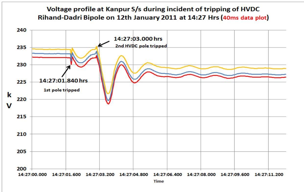
Figure 56: Dip and rise in voltage profile at Kanpur
