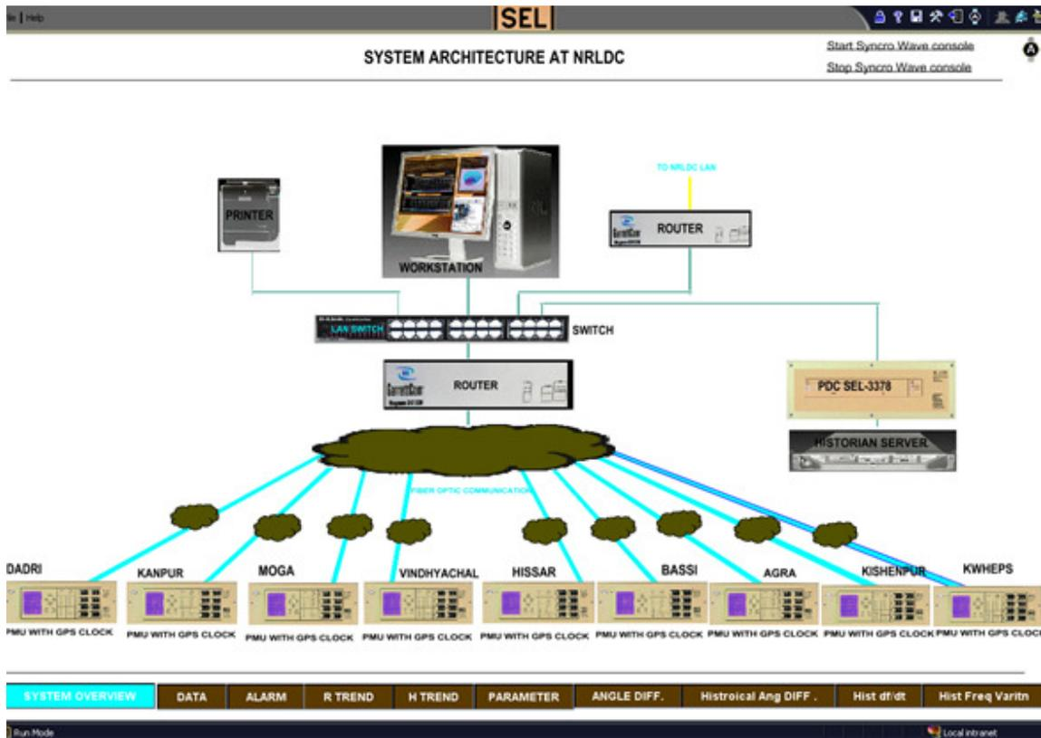
Figure 16: Architecture of pilot project in Northern Region
