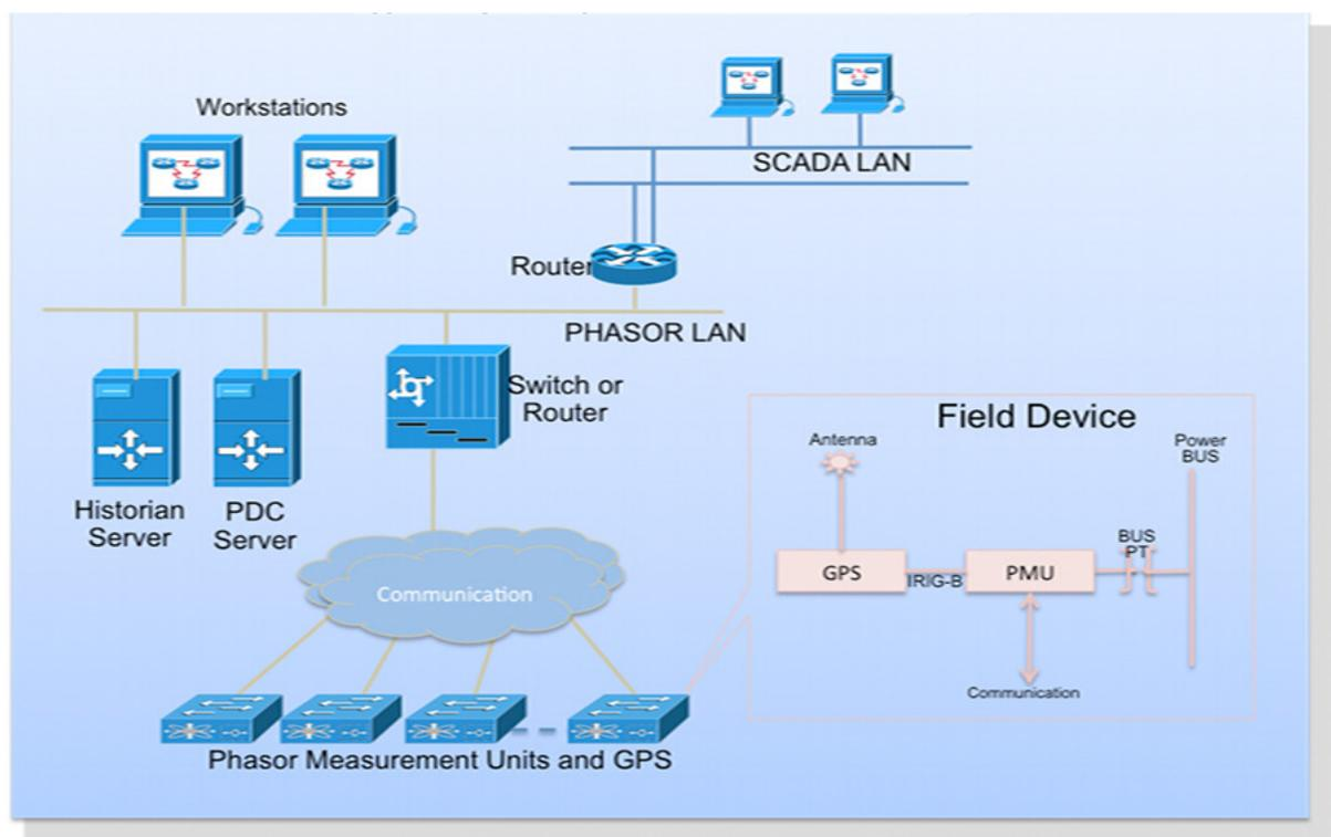
Figure 10: General architecture of a Synchrophasor project
