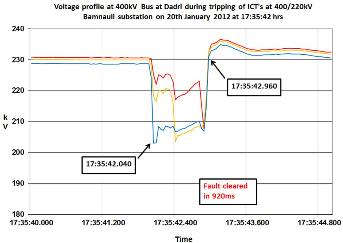
Figure 54: Voltage profile at Dadri indicating possible operation of back up protection
