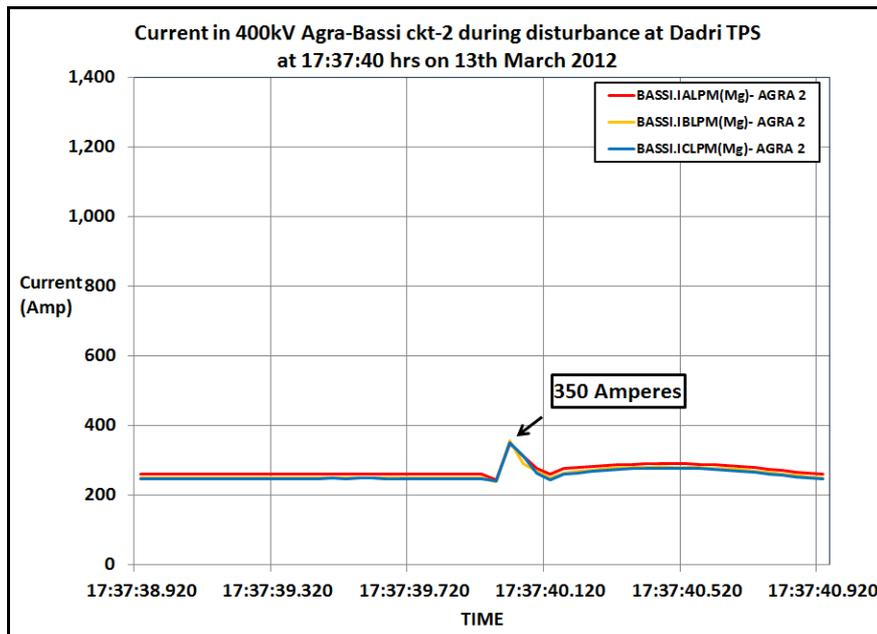
Figure 87: Current flow in 400kV Agra-Bassi line -2
