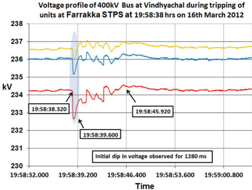
Figure 58: Voltage profile at Vindhyachal (NR) during tripping of units at Farakka STPS (ER)
