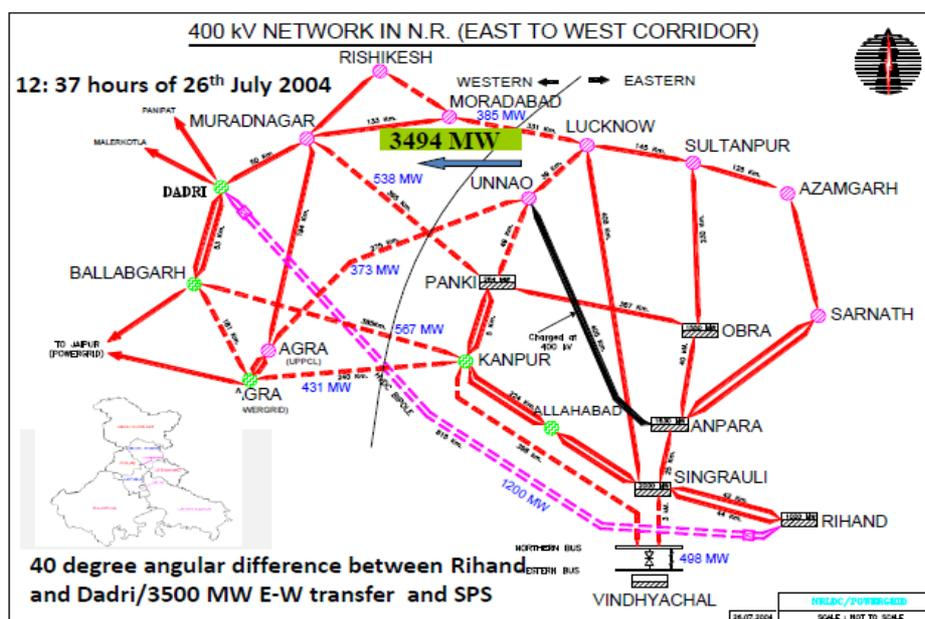
Figure 2: Angular separation between Rihand and Dadri on 26-July-2004
