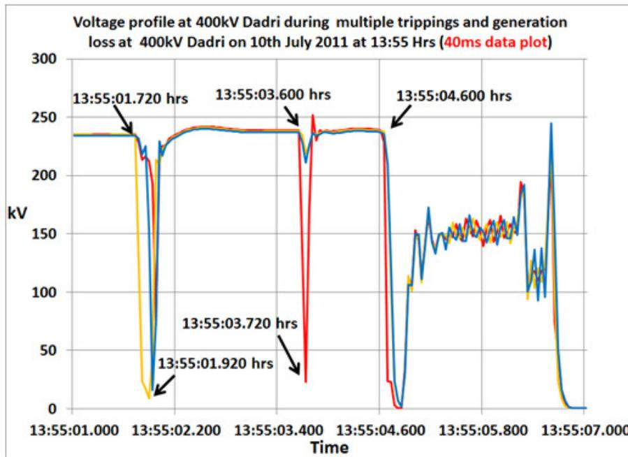
Figure 80: Fluctuations in voltage at Dadri during generation loss at Dadri on 10th July 2011
