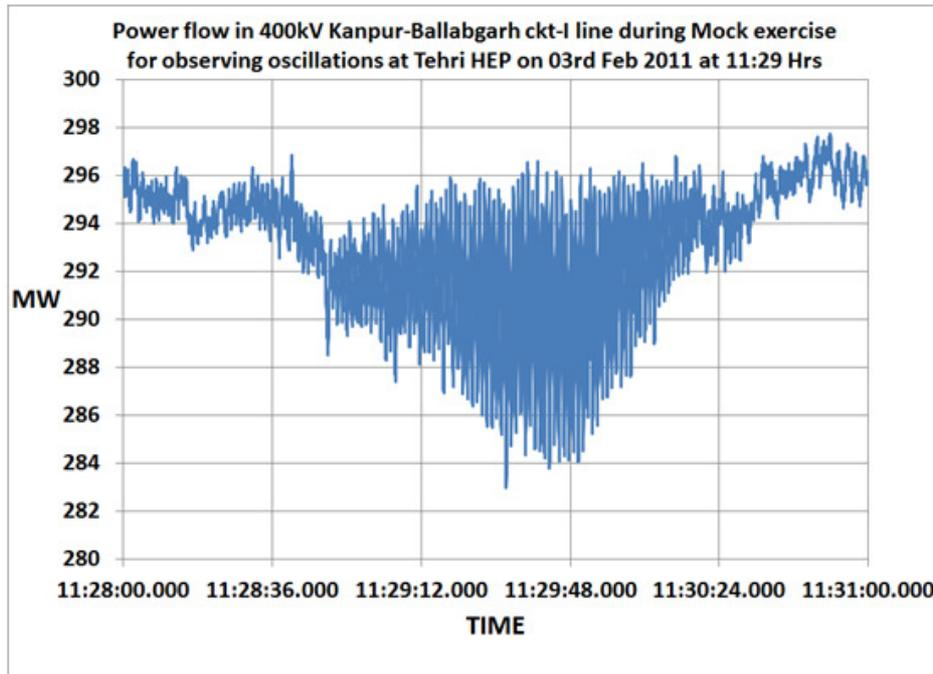
Figure 95: Oscillations in Kanpur-ballabgarh flow due to increased flow in Tehri-Meerut
