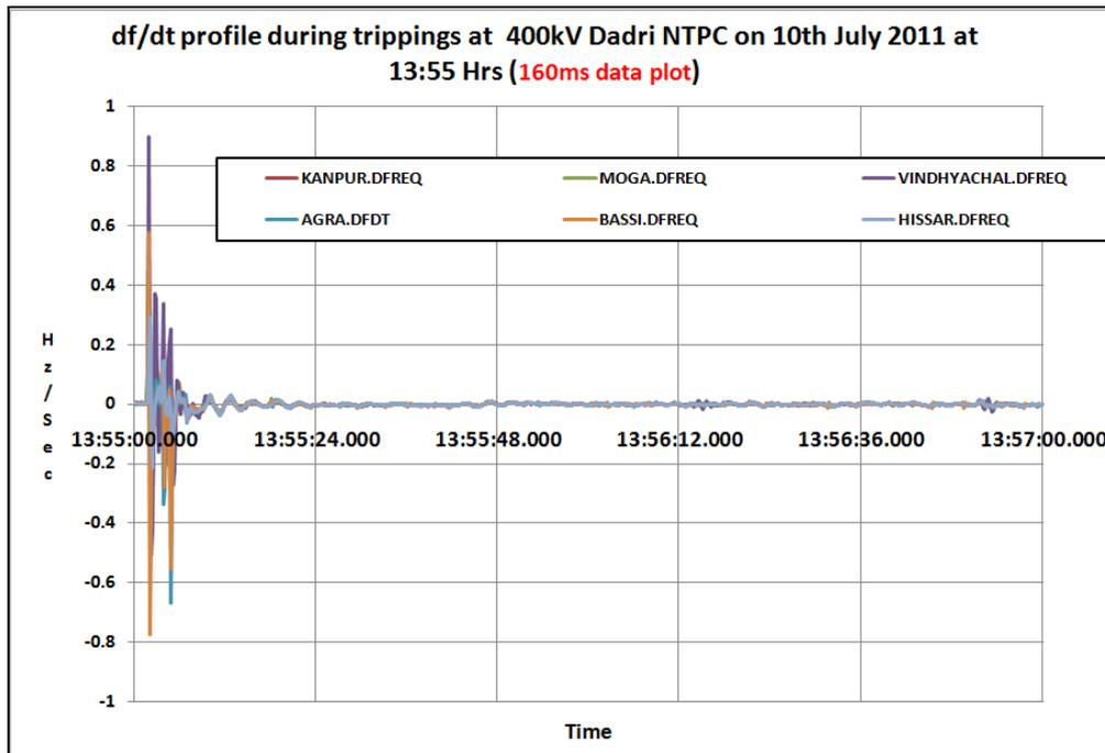
Figure 129: df/dt profile during tripping of Dadri NTPC on 19th July 2011
