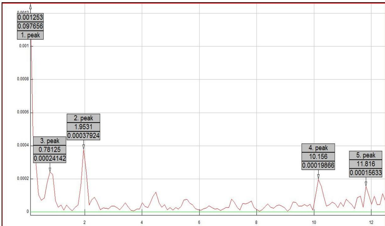
Figure 121: FFT of the frequency at Raipur ( HVDC flow is 900 MW)
