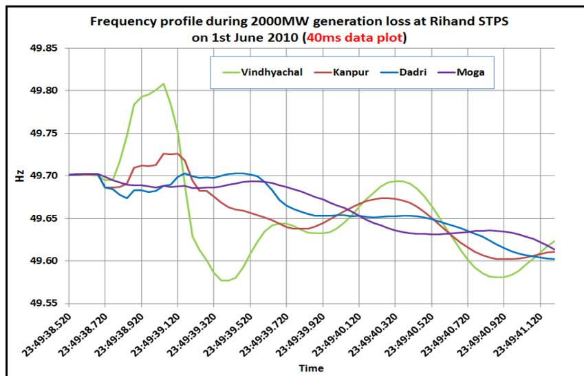
Figure 105: Swing in frequency during generation loss at Rihand STPS
