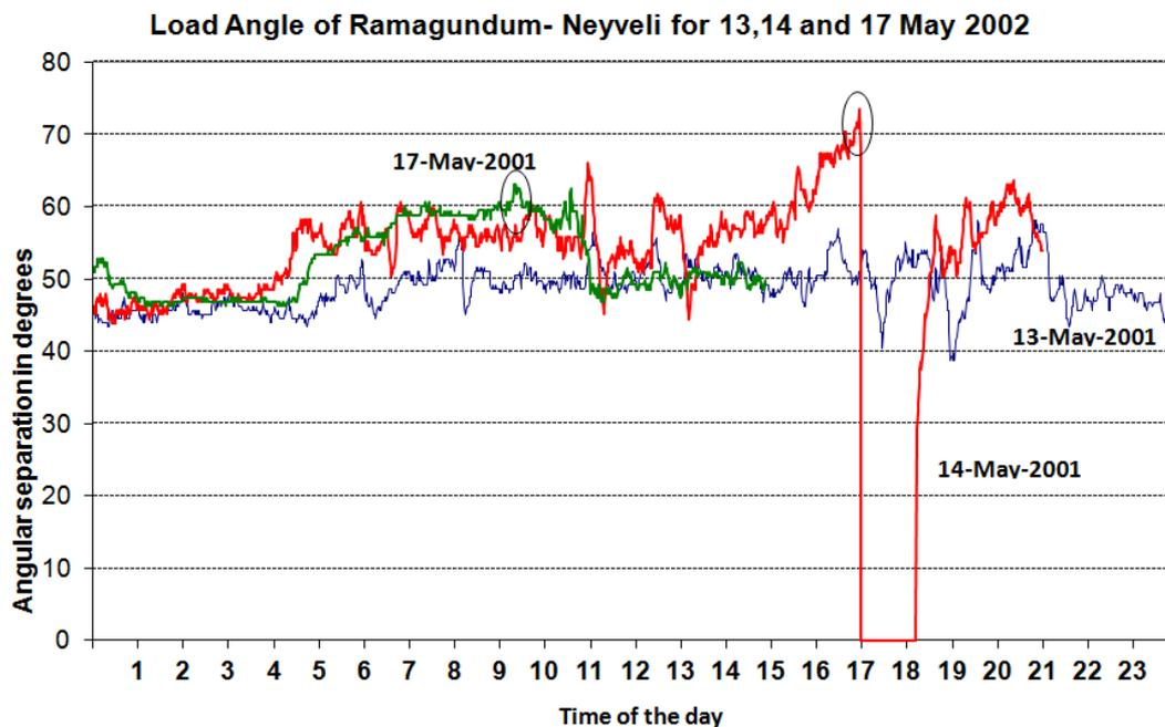
Figure 1: Load angle between Ramagundam and Neyveli for 13, 14 and 17 May 2002
