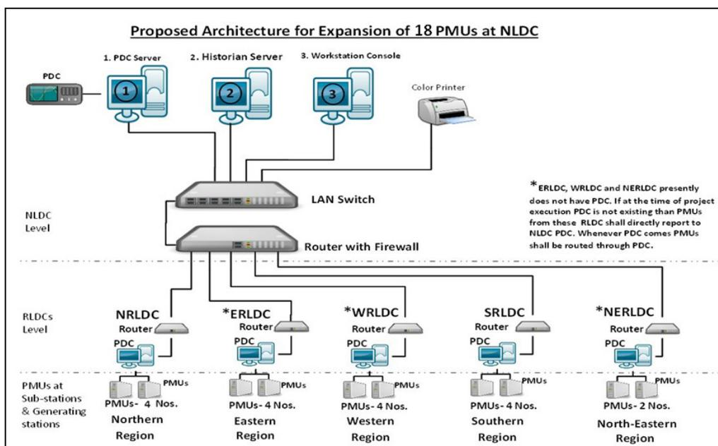
Figure 12: Proposed architecture for Phase-III of PMU pilot project in NR
