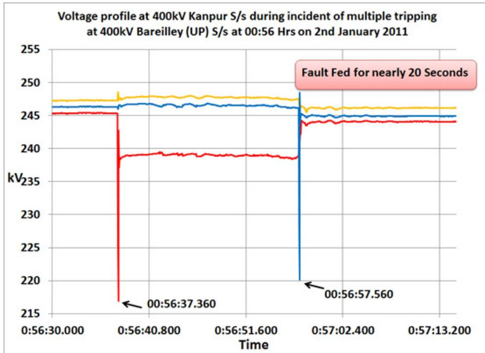
Figure 78: Voltage profile of Kanpur bus showing a high resistance fault at 400kV Bareilly UP
