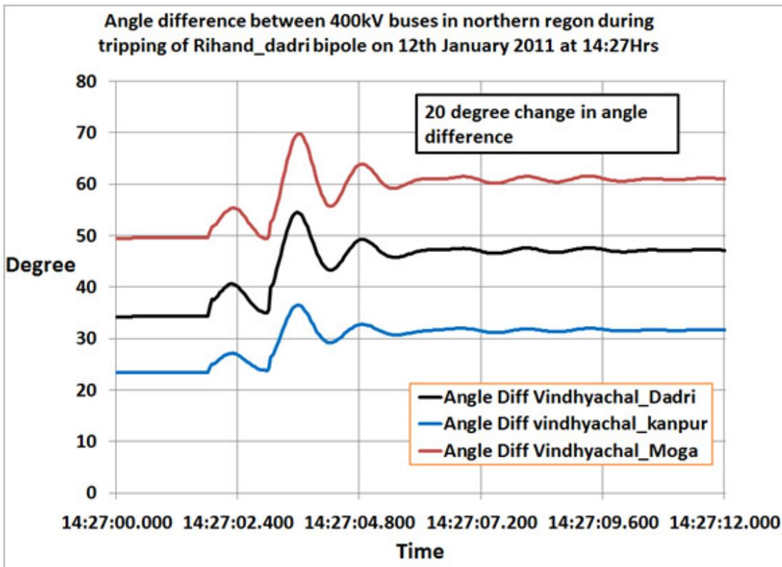
Figure 83: Angular swing observed on tripping of HVDC Rihand Dadri bipole
