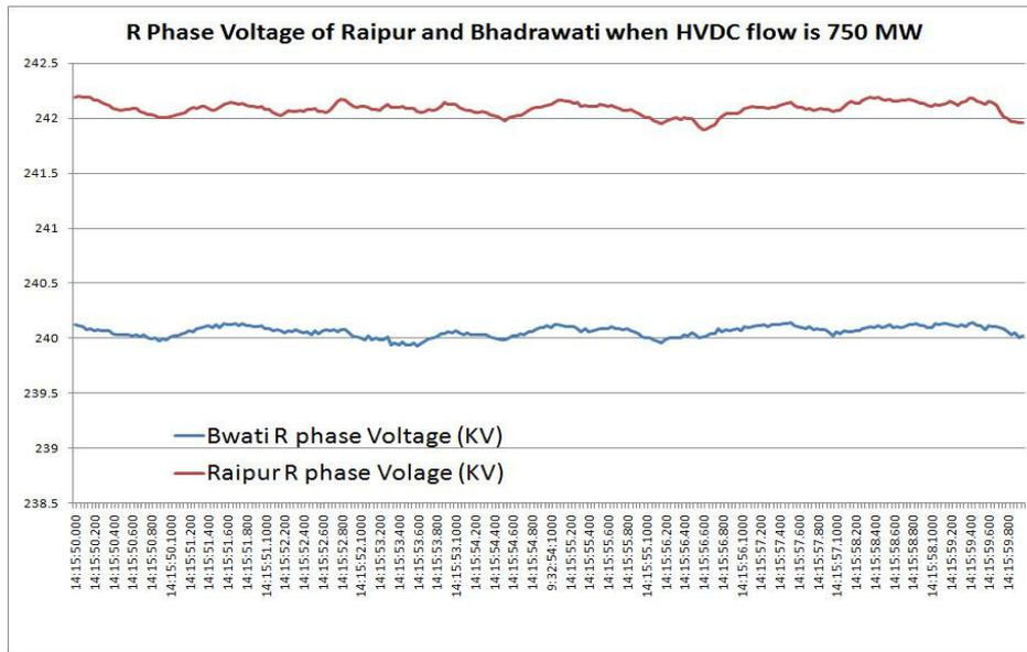
Figure 109: R phase voltage of Raipur and Bhadrawati when HVDC flow is 750 MW
