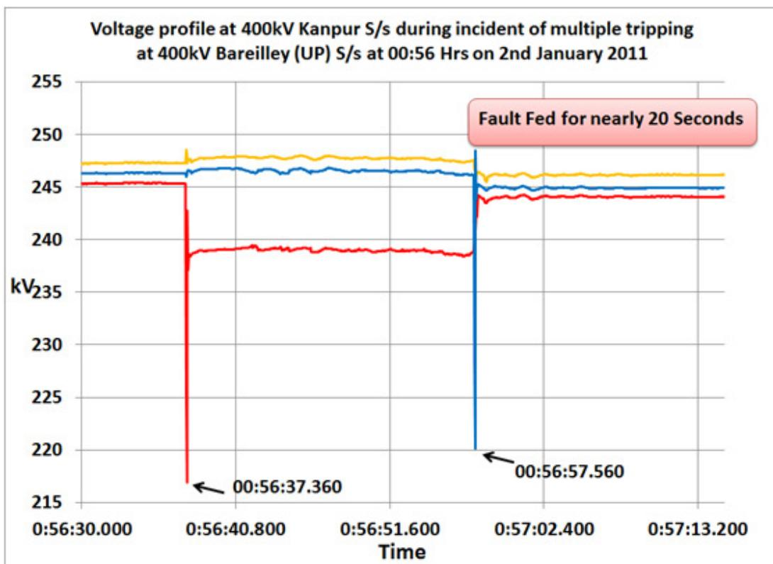
Figure 55: Voltage profile at Kanpur showing delayed clearance of fault
