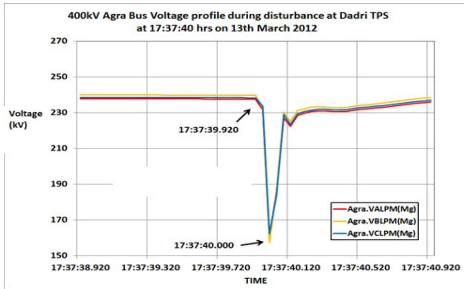
Figure 48: Dip in phase voltage at 400 kV Agra during 3 phase fault at 400 kV Dadri
