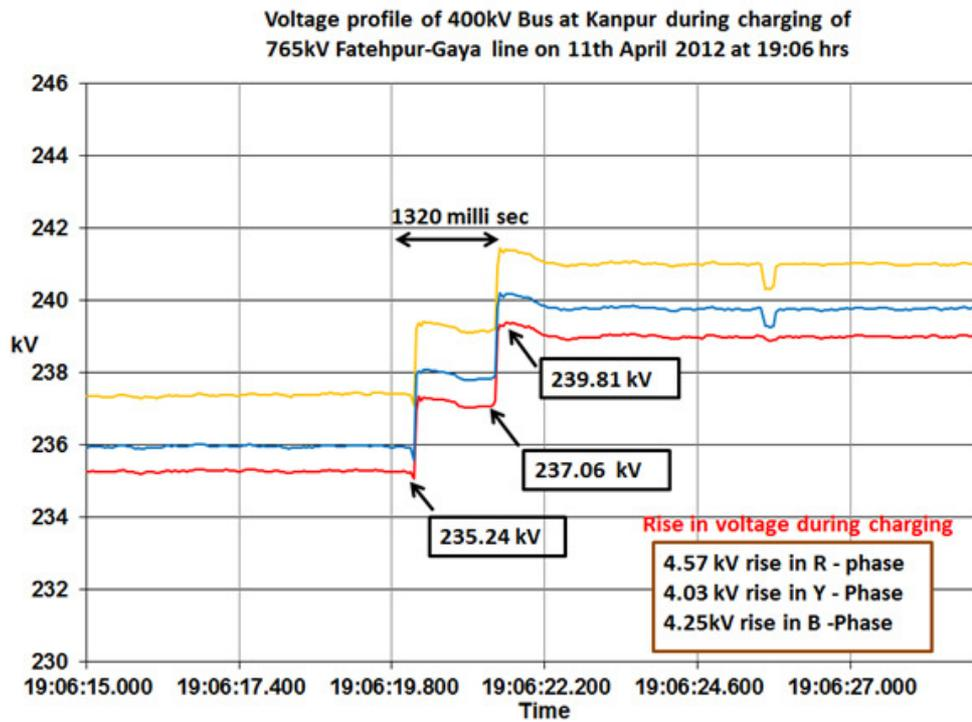
Figure 67: Zoom in voltage at 400 kV Kanpur during charging of 765 kV Fatehpur-Gaya
