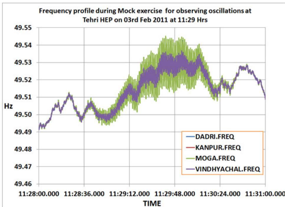
Figure 96: Oscillations observed in frequency during increase in flow on Tehri-Meerut
