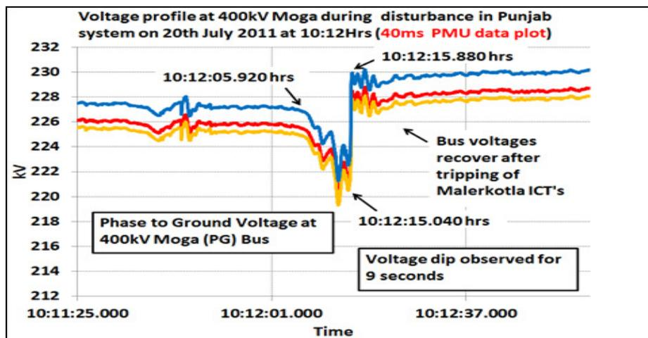
Figure 59: Dip in voltage at Moga during disturbance in Punjab system
