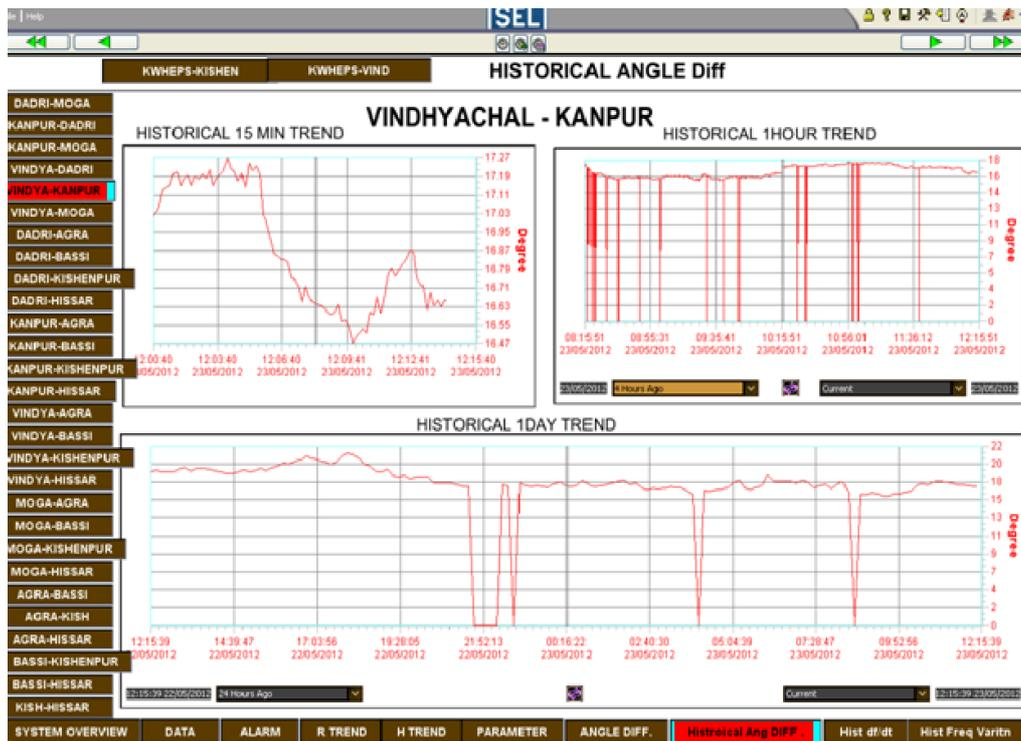
Figure 25: Trends display of angle difference between 400kV buses
