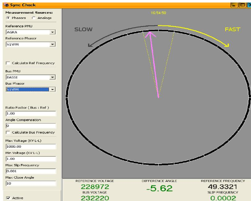
Figure 23: Dial display of opposite voltage phasors used for synchronising check
