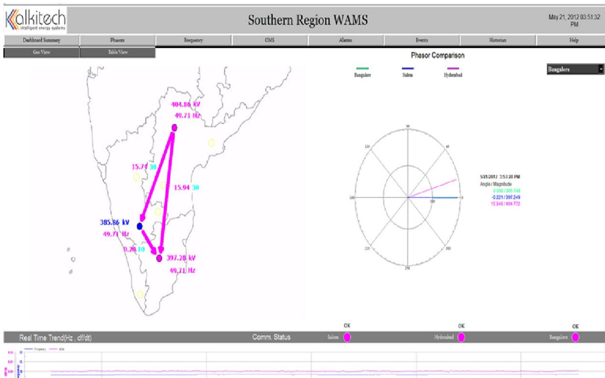
Figure 38: Dial display of angular separation
