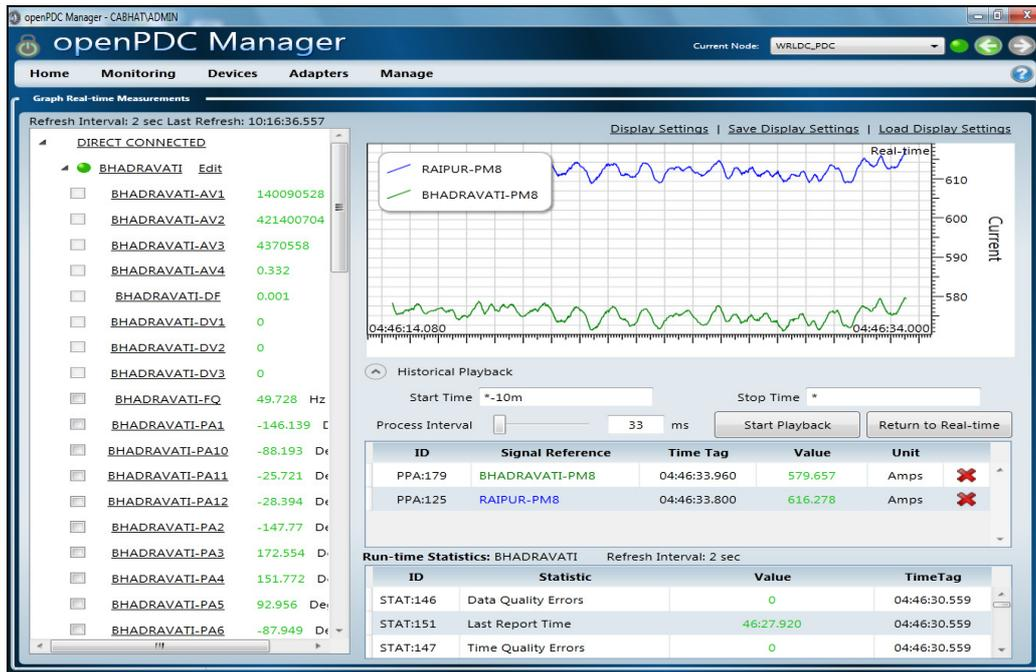
Figure 33: Real time PMU data visualisation window in openPDC
