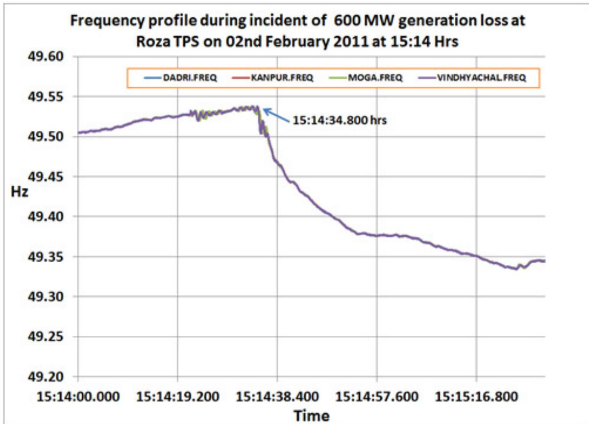
Figure 63: Fall in frequency during 600 MW generation loss at Rosa TPS
