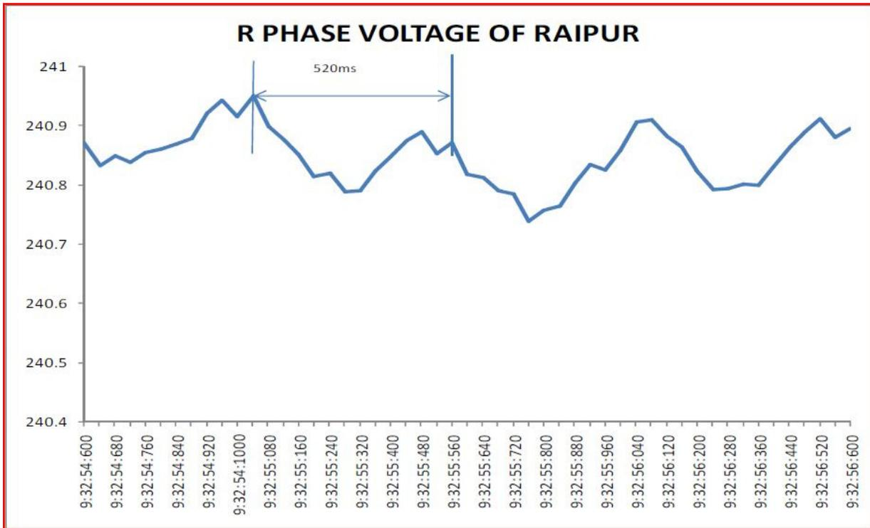
Figure 114: R phase voltage at Raipur showing frequency of oscillations
