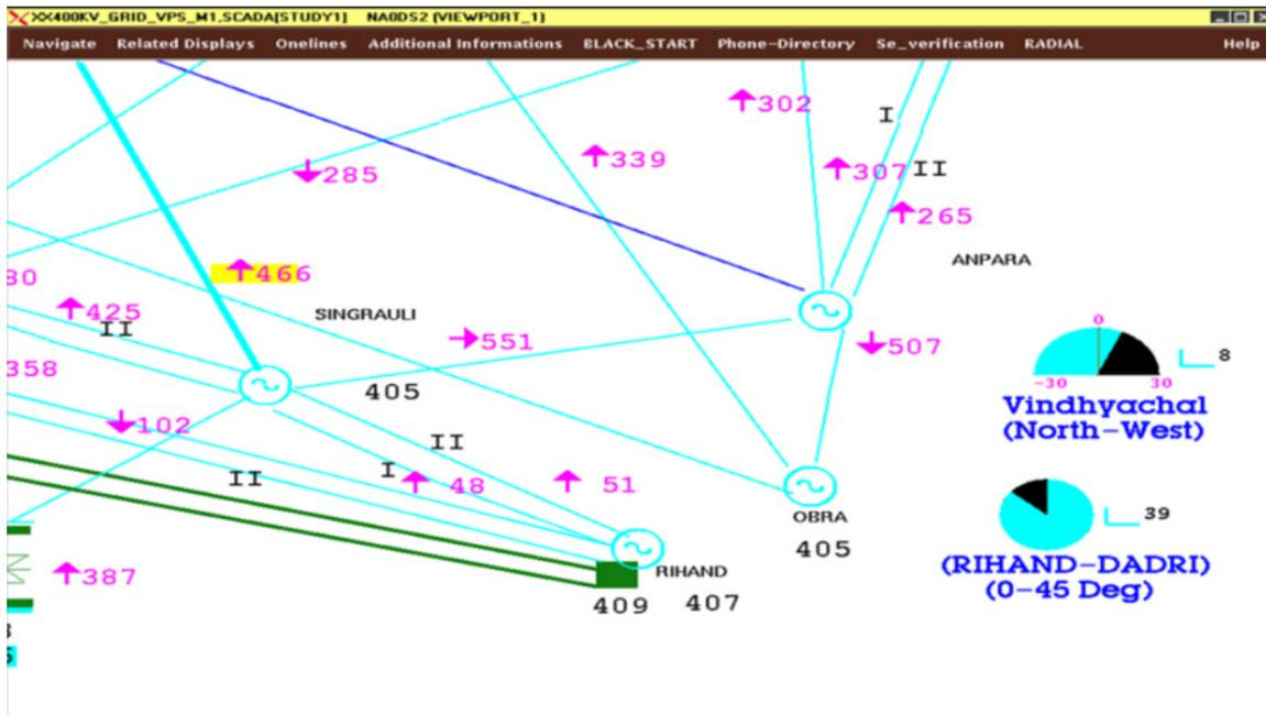
Figure 3: Monitoring of angular separation between Rihand and Dadri
