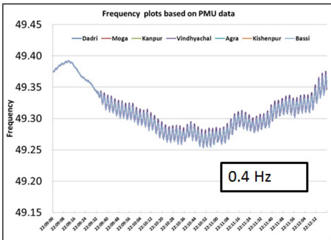
Figure 98: Low frequency oscillations in Dadri frequency
