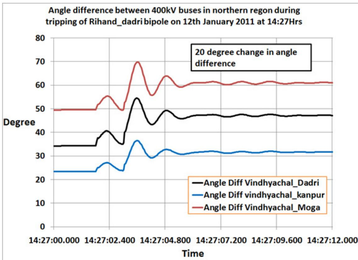
Figure 45: Angular difference during tripping of Rihand Dadri bipole
