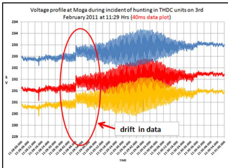
Figure 132: Drift seen in voltage plot during oscillations on 3rd February 2011
