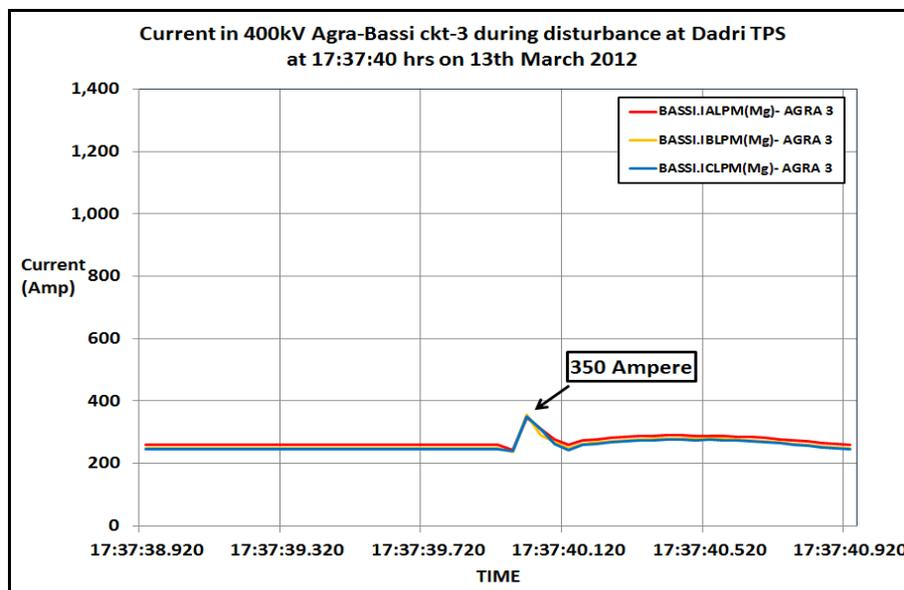
Figure 88: Current flow in 400kV Agra-Bassi line -3
