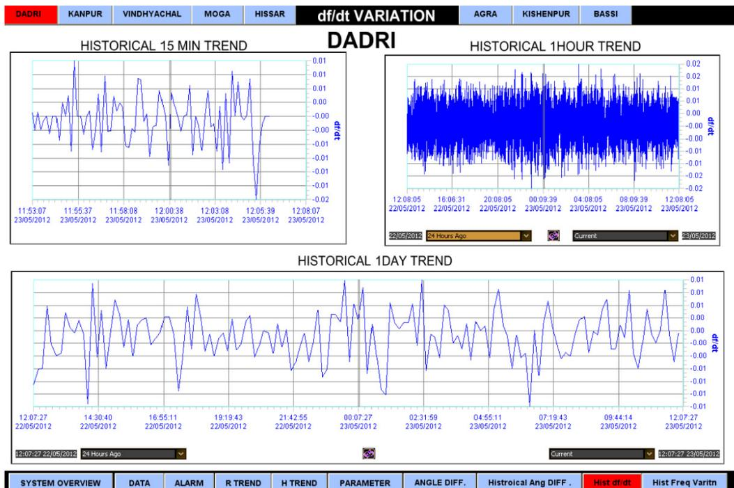
Figure 26: Trends display of rate of change of frequency recorded at 400kV Dadri bus
