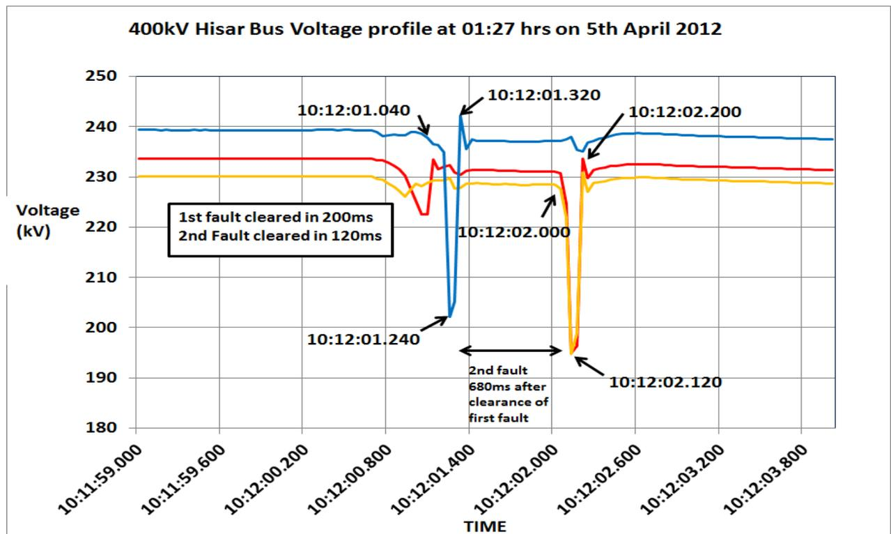
Figure 51: Voltage profile corroborating the fault clearance time at Hissar
