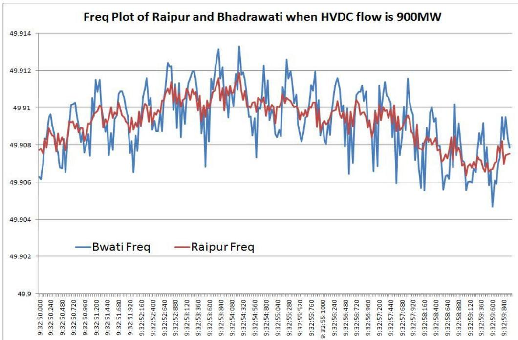
Figure 112: Oscillations in frequency when power flow on HVDC Bhadrawati is 900 MW
