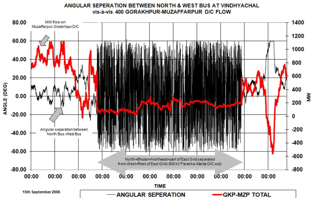
Figure 4: Detection of islanding in a synchronous grid (15-Sep-2006)
