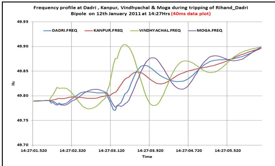
Figure 104: Swing in frequency during tripping of Rihand-Dadri bipole
