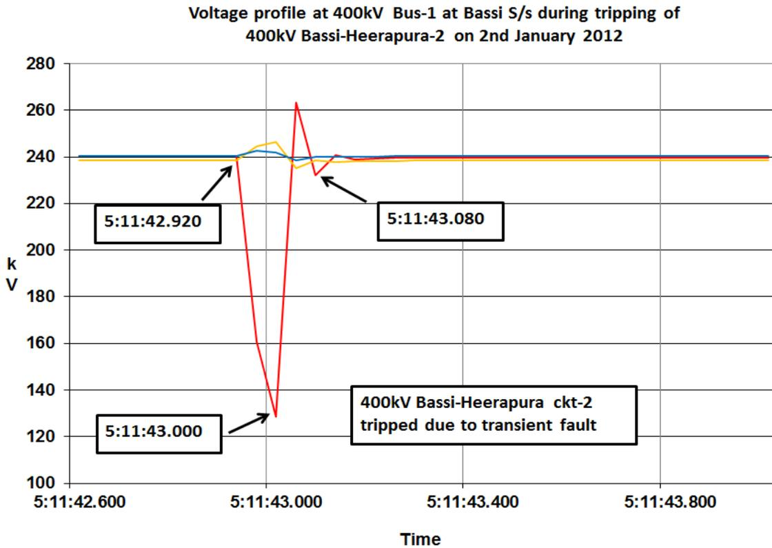
Figure 50: Dip in R phase voltage at Bassi during tripping of 400 kV Bassi-Heerapura II
