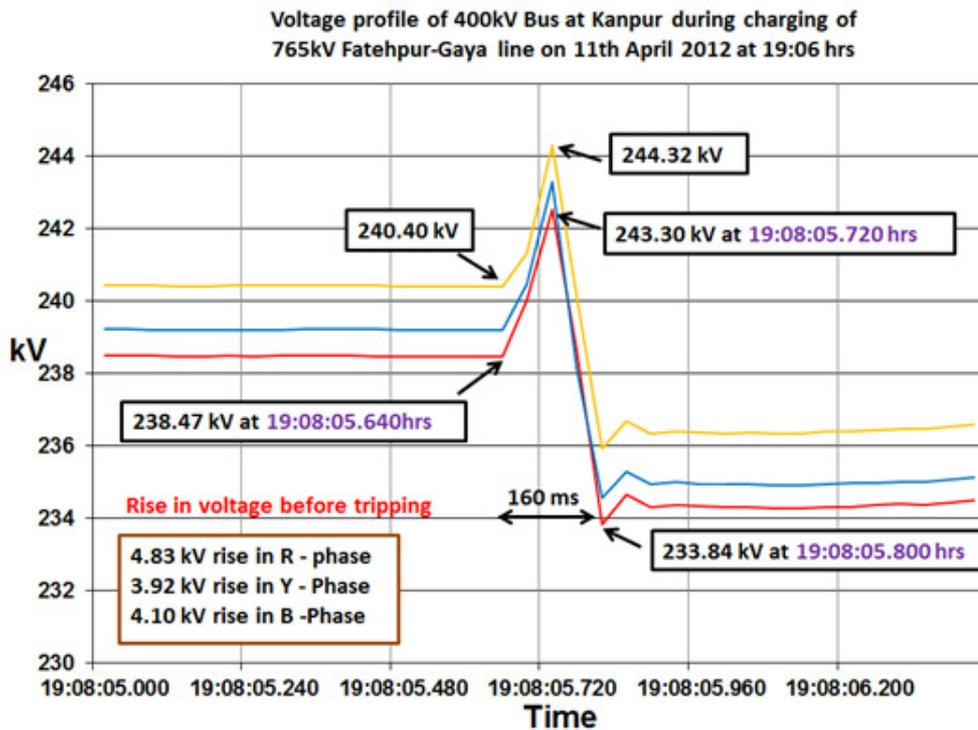
Figure 68: Zoom in of voltage at 400 kV Kanpur during charging of 765 kV Fatehpur-Gaya
