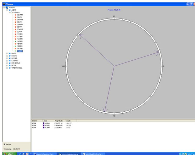
Figure 22: Dial type display of voltage phasors
