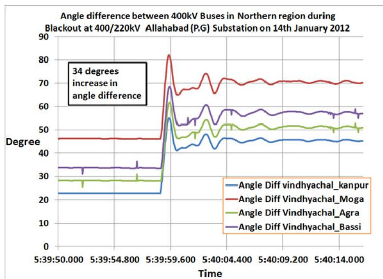
Figure 44: Angular difference between buses in NR during blackout at 400 kV Allahabad
