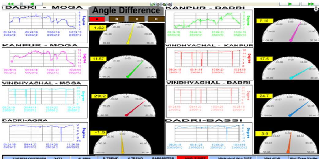
Figure 24: Trend and dial type display for angle difference between different 400kV buses
