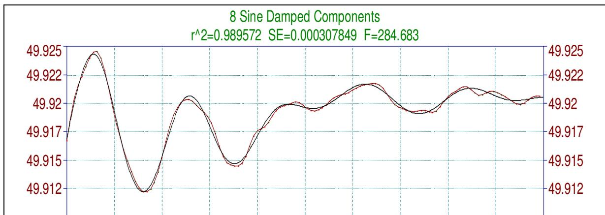
Figure 126: Prony Analysis of Frequency using 8 exponentially sine damped case
