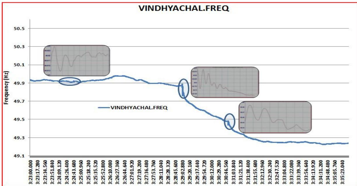
Figure 124: PMU plot for Vindhyachal frequency showing the three incidences
