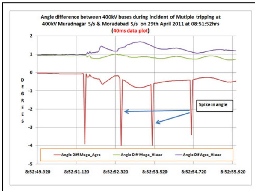
Figure 133: Spikes seen in angular difference during a grid event
