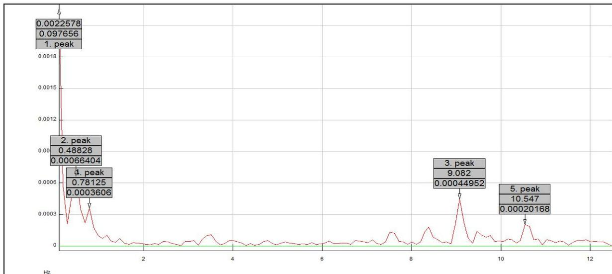
Figure 115: FFT of frequency at Bhadrawati (HVDC B'wati flow 750MW)
