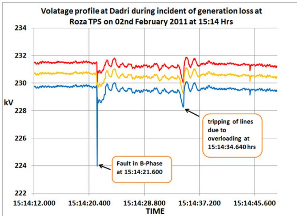
Figure 62: Dip in voltage at Dadri during generation loss at Roza TPS
