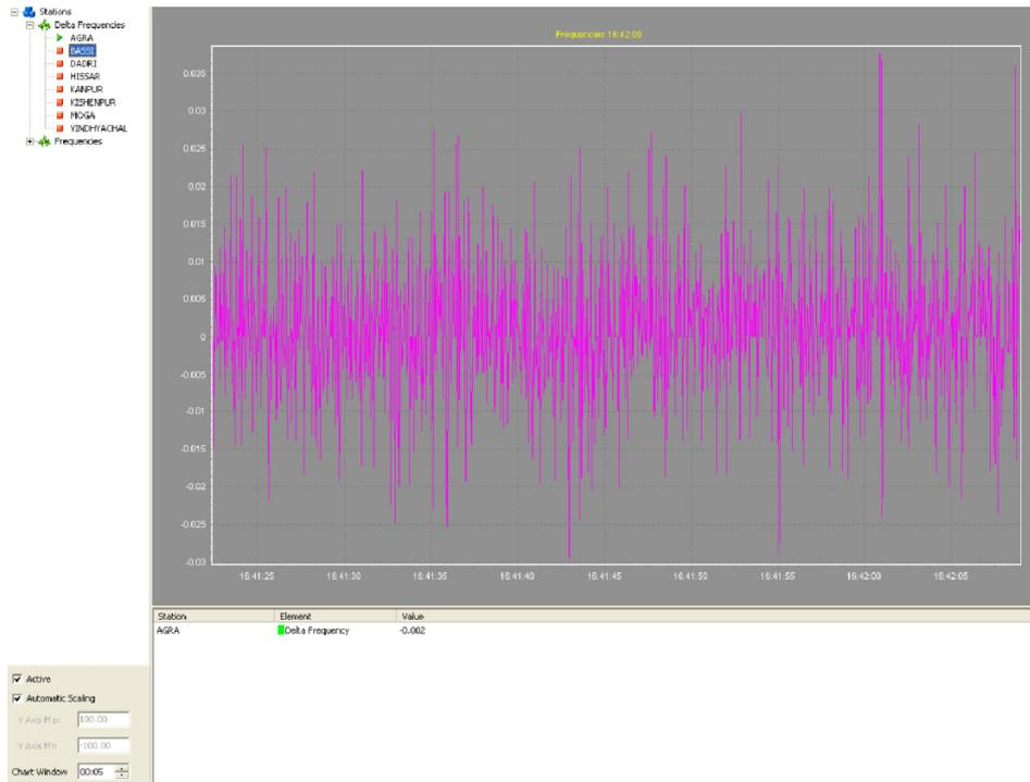
Figure 19: Trend display of the rate of change of frequency
