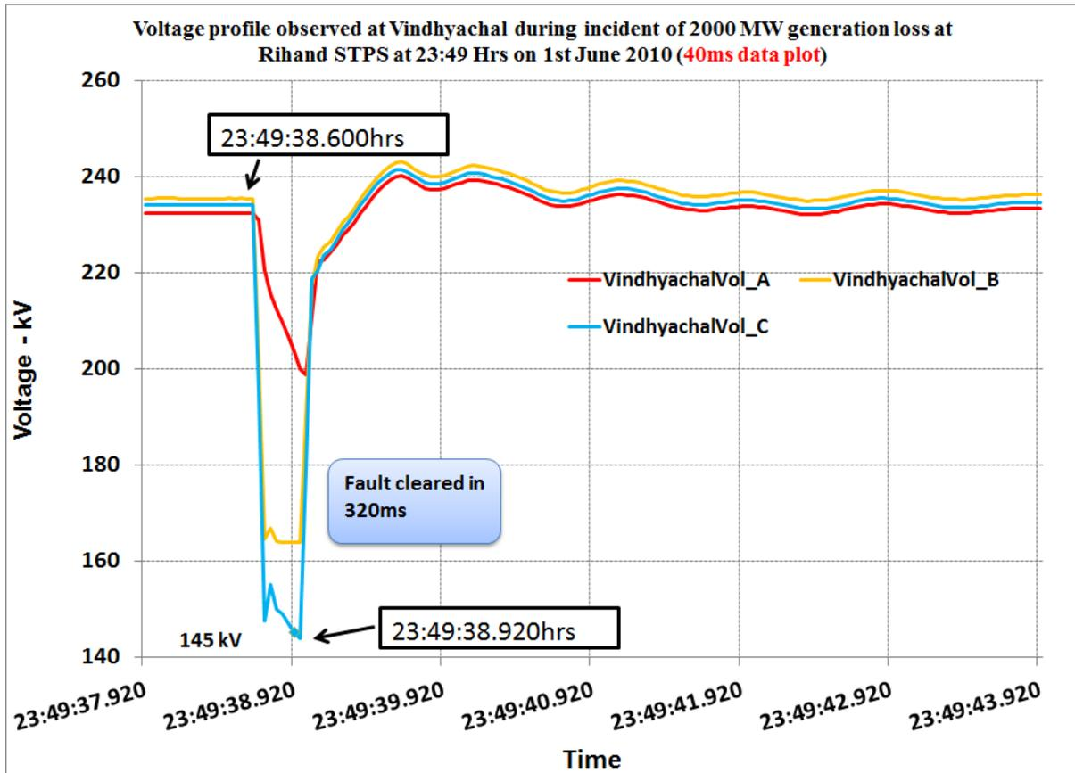
Figure 53: Voltage profile at Vindhyachal indicating the probable operation of LBB protection
