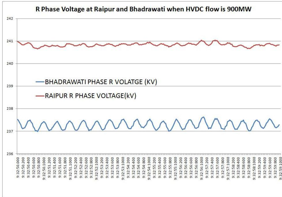
Figure 111: Oscillations seen in Raipur and Bhadrawati when HVDC flow is 900 MW
