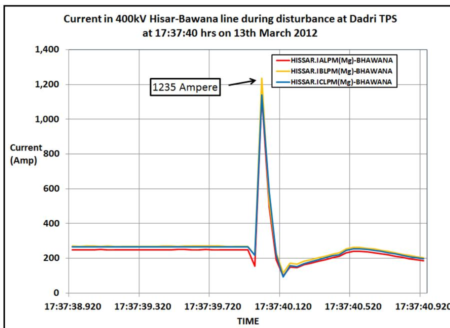
Figure 89: current flow in 400kV Hisar-Bawana line
