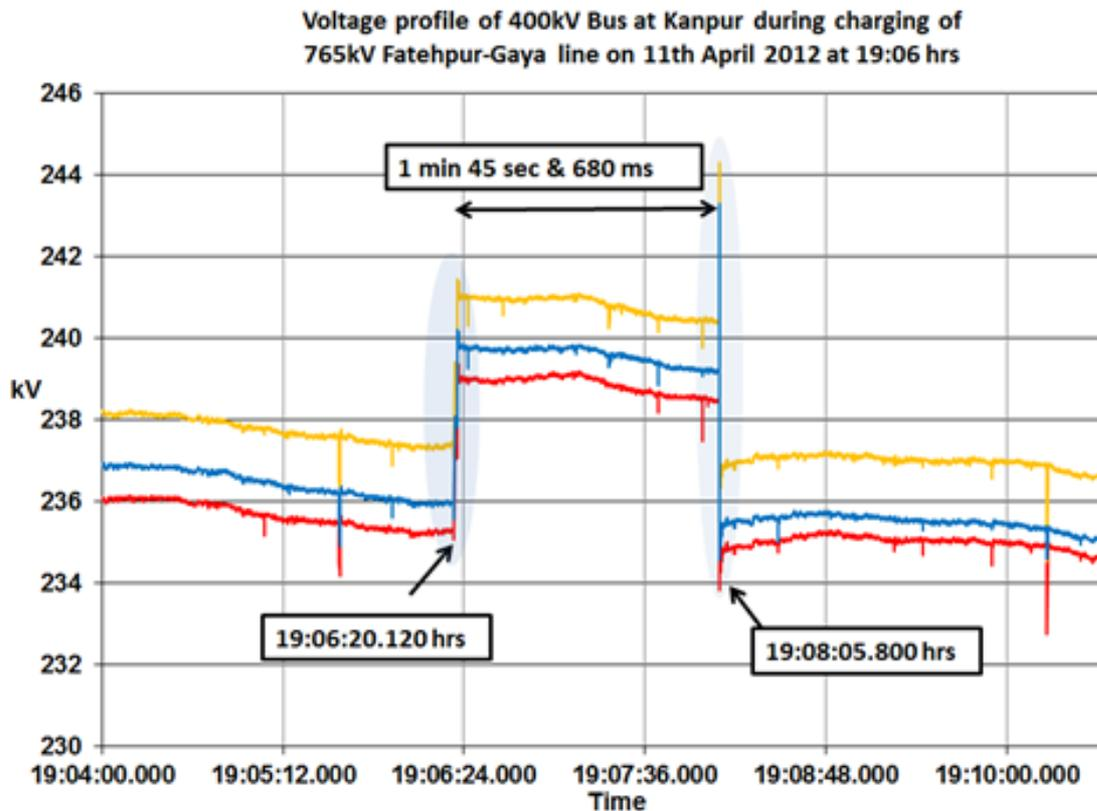
Figure 66: Voltage at 400 kV Kanpur during charging of 765 kV Fatehpur-Gaya
