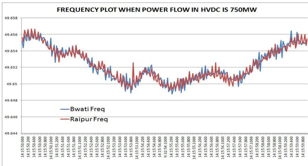
Figure 110: Frequency plot when power flow on HVDC Bhadrawati is 750 MW
