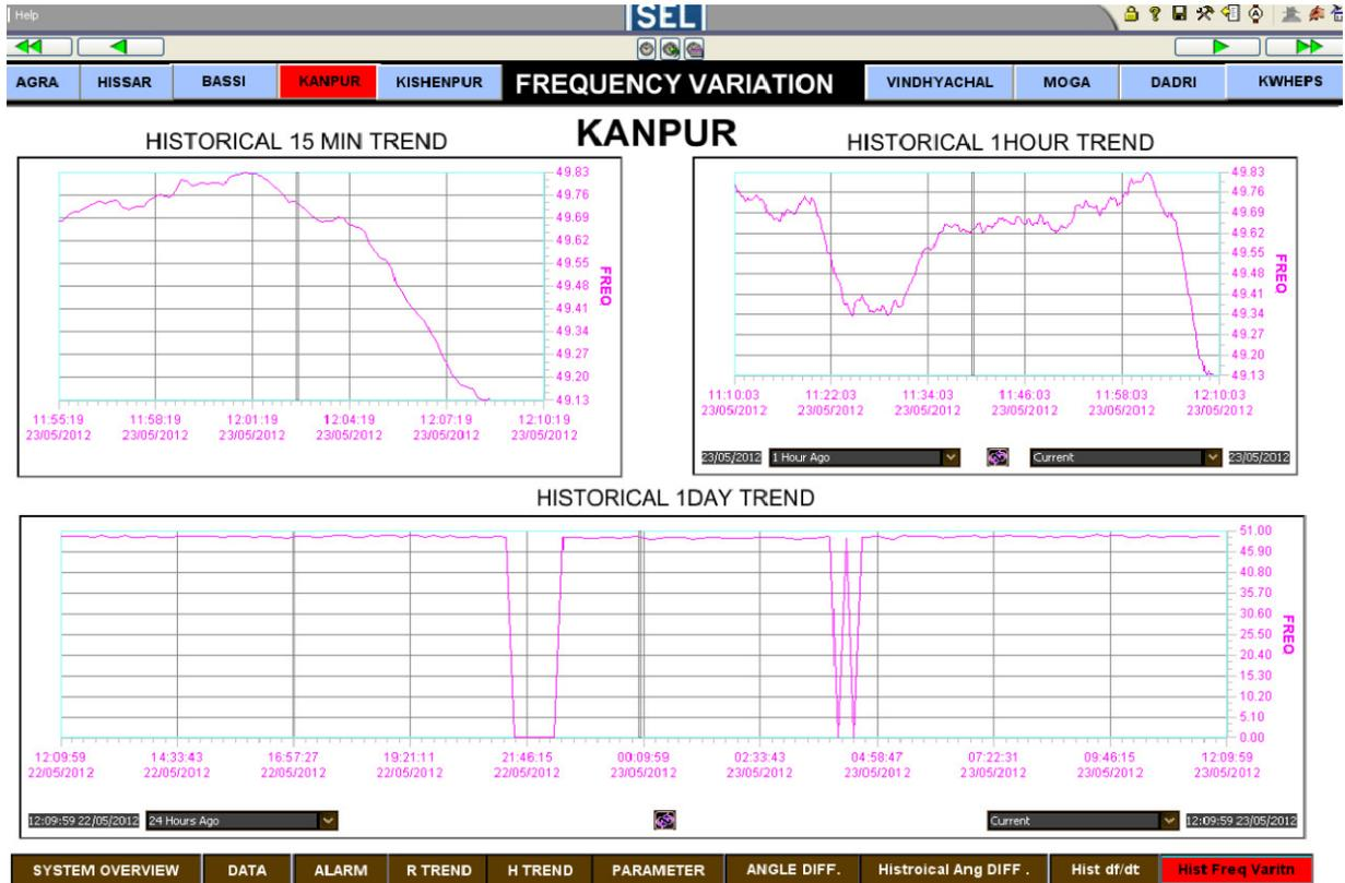
Figure 27: Trend display of frequency profile recorded at 400kV Kanpur bus
