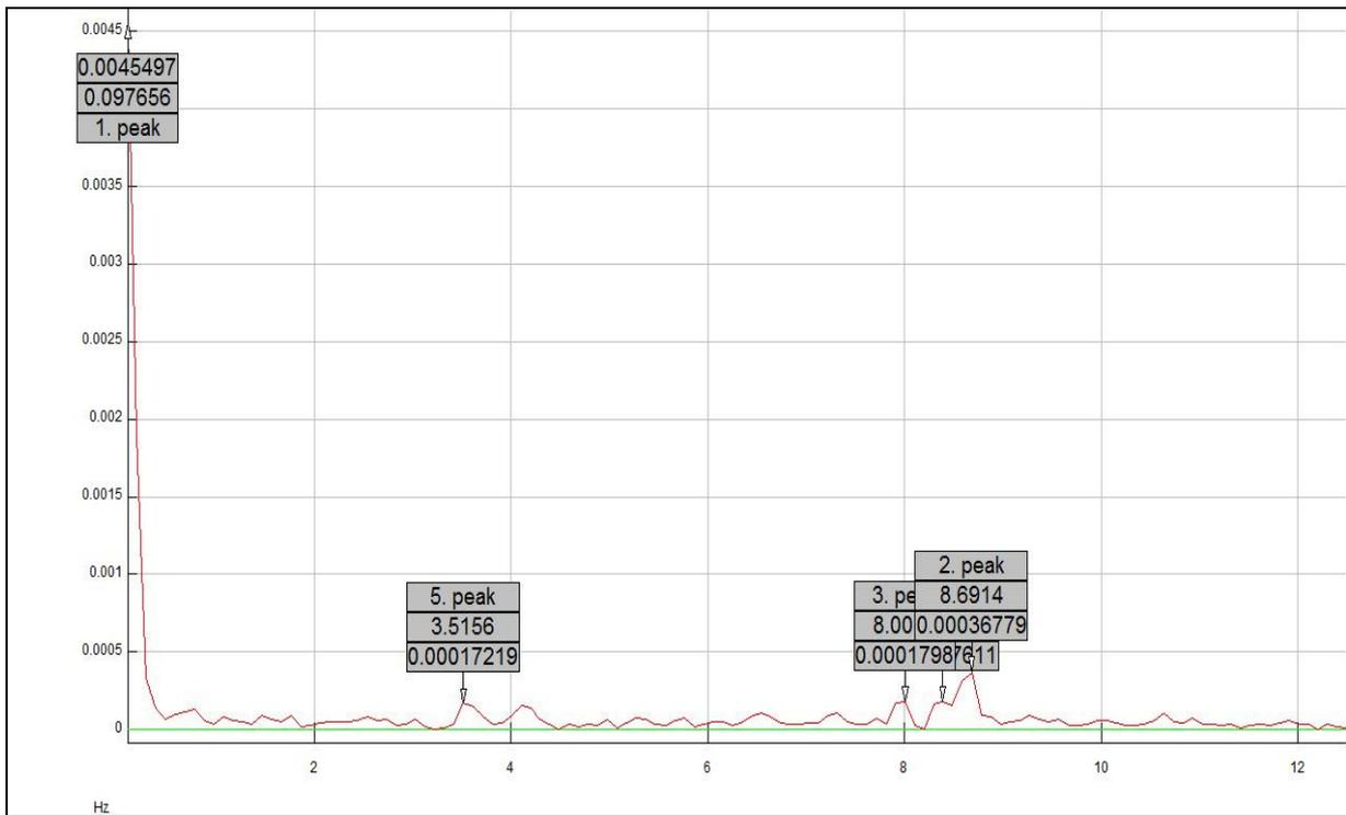
Figure 118: FFT of the frequency at Bangalore (HVDC B'wati flow is 750MW)
