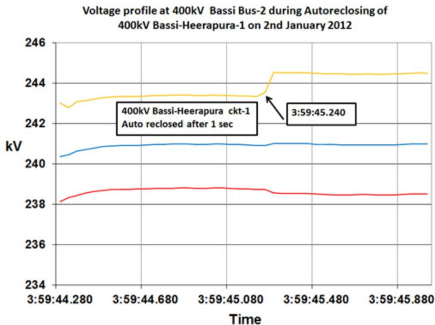
Figure 70: Rise in Bassi Y-ph voltage during auto-reclose of 400 kV Bassi-Heerapura
