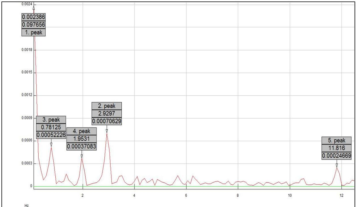
Figure 123: FFT of the frequency at Bengaluru ( HVDC flow is 900 MW)
