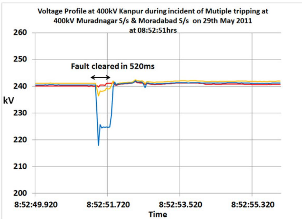
Figure 52: Detection of delayed fault clearance
