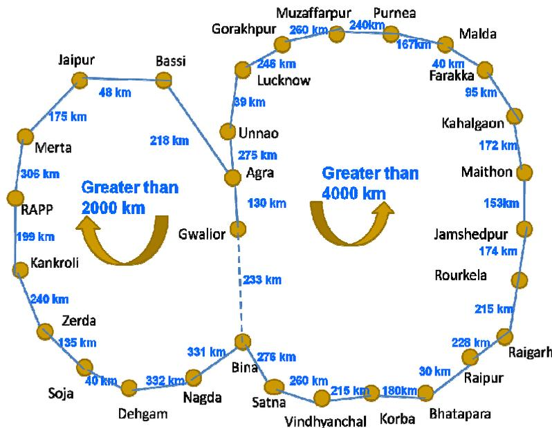
Figure 6: Diversion of power after tripping of 400 kV Bina-Gwalior (28-Nov-2009)
