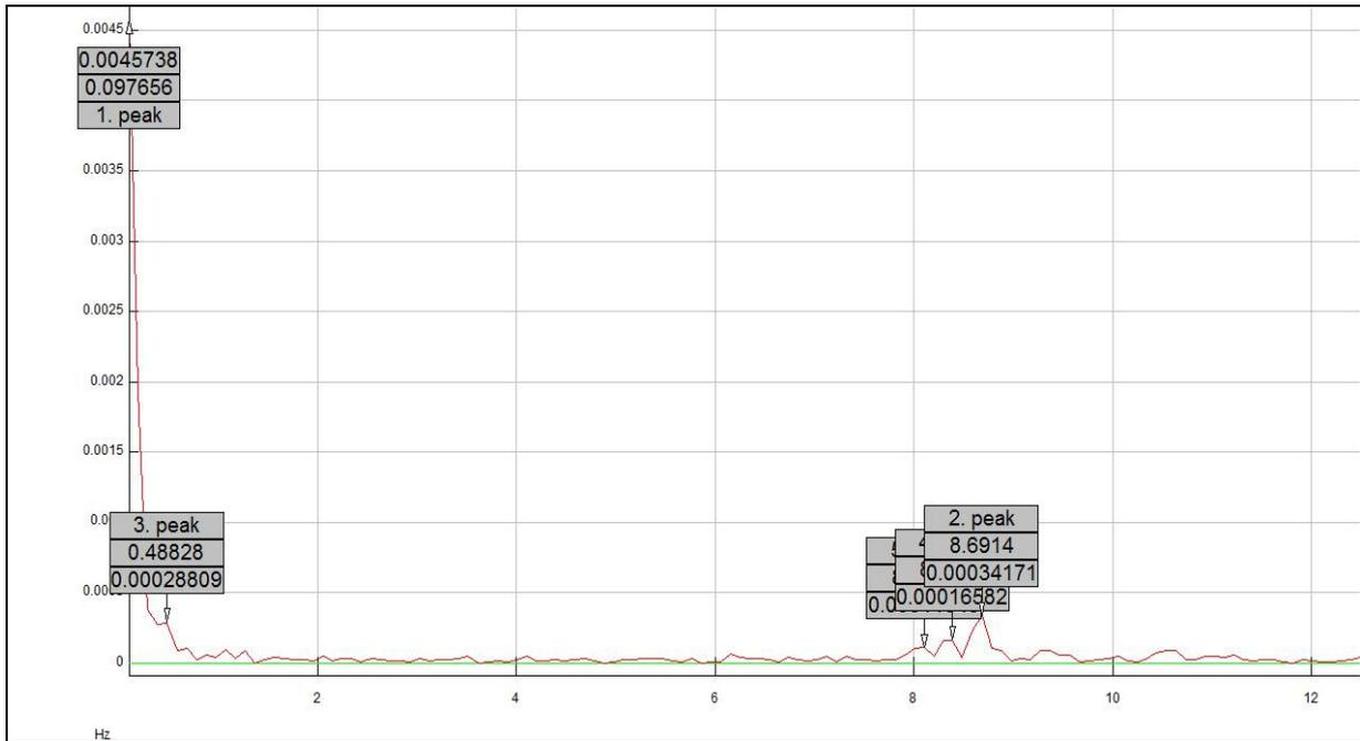
Figure 117: FFT of frequency at Hyderabad (HVDC B'wati flow 750MW)
