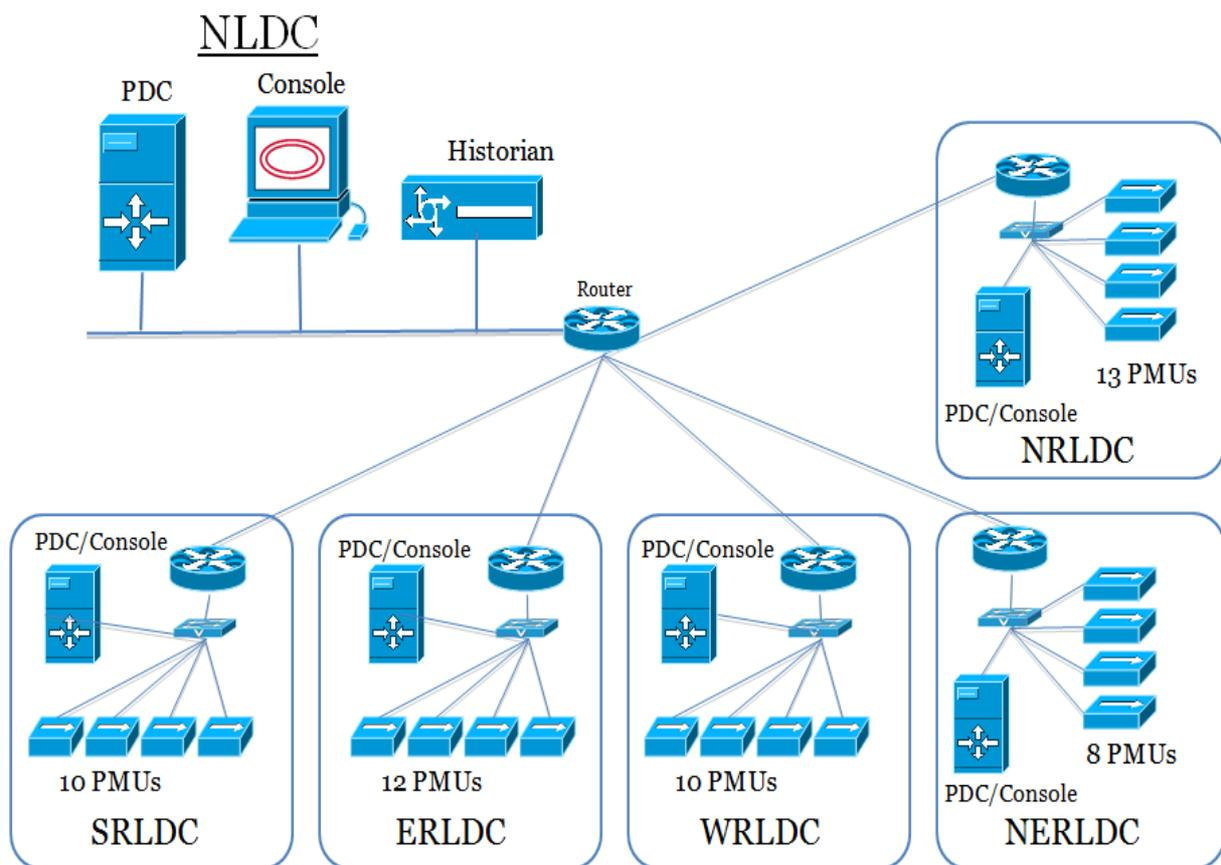
Figure 14: Envisaged architecture after completion of the pilot projects in all the Regions
