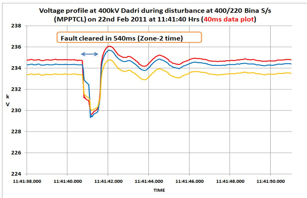
Figure 57: Dip in 3-phase voltage seen in Dadri (NR) during fault at 400 kV Bina (WR)
