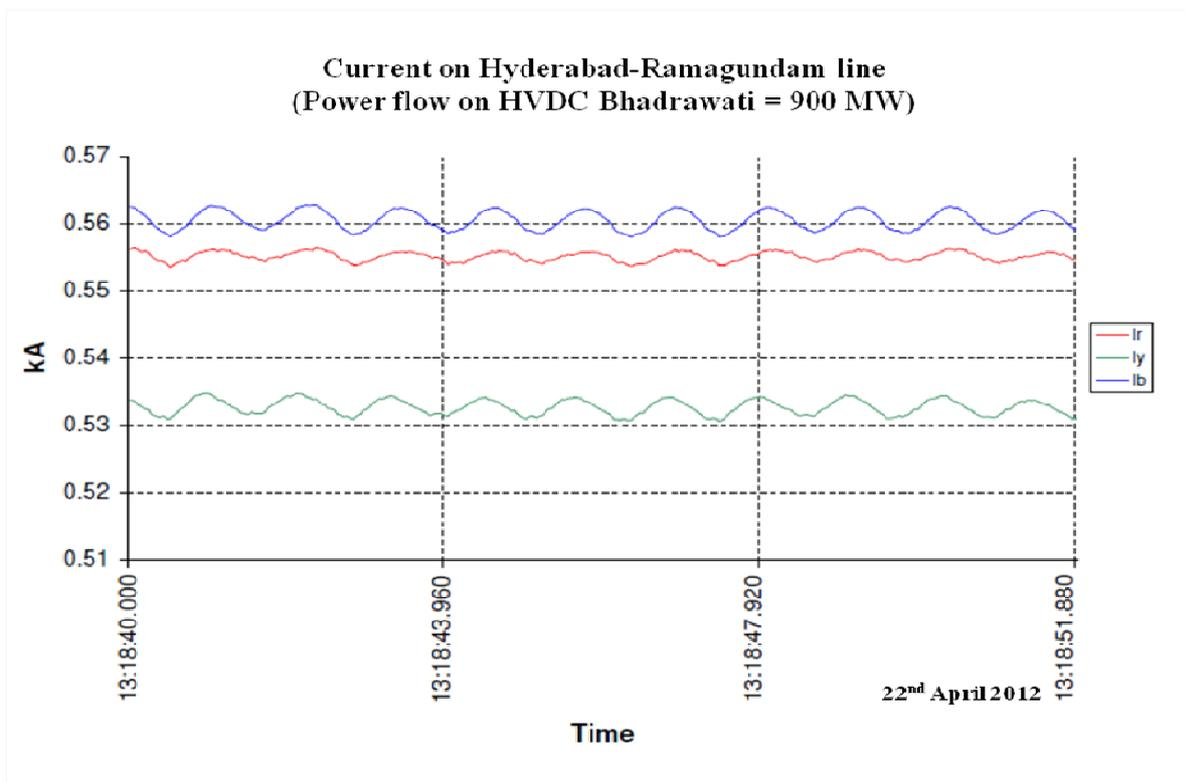
Figure 108: Flow on Hyderabad-Ramagundam (HVDC Bhadrawati = 900 MW)
