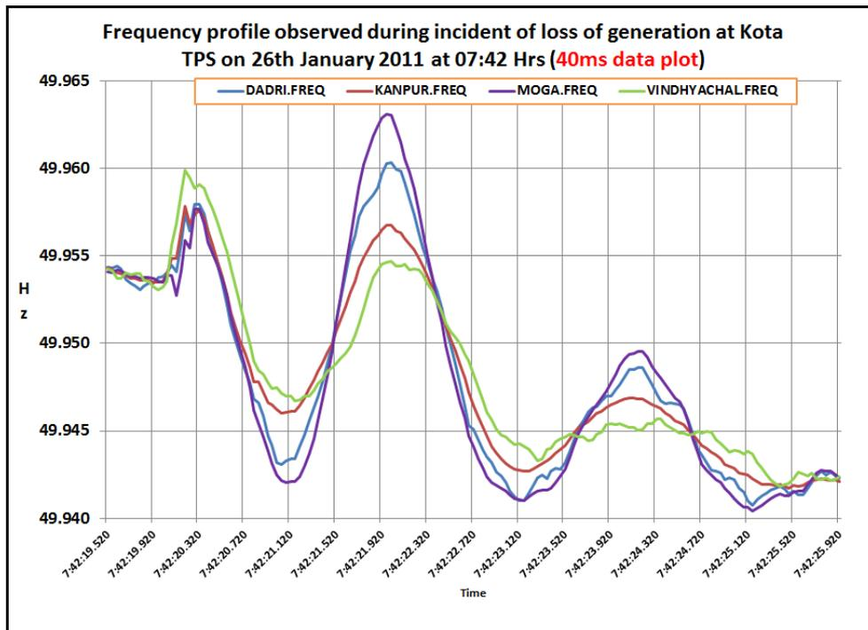
Figure 106: Swing in frequency profile during generation loss at Kota TPS
