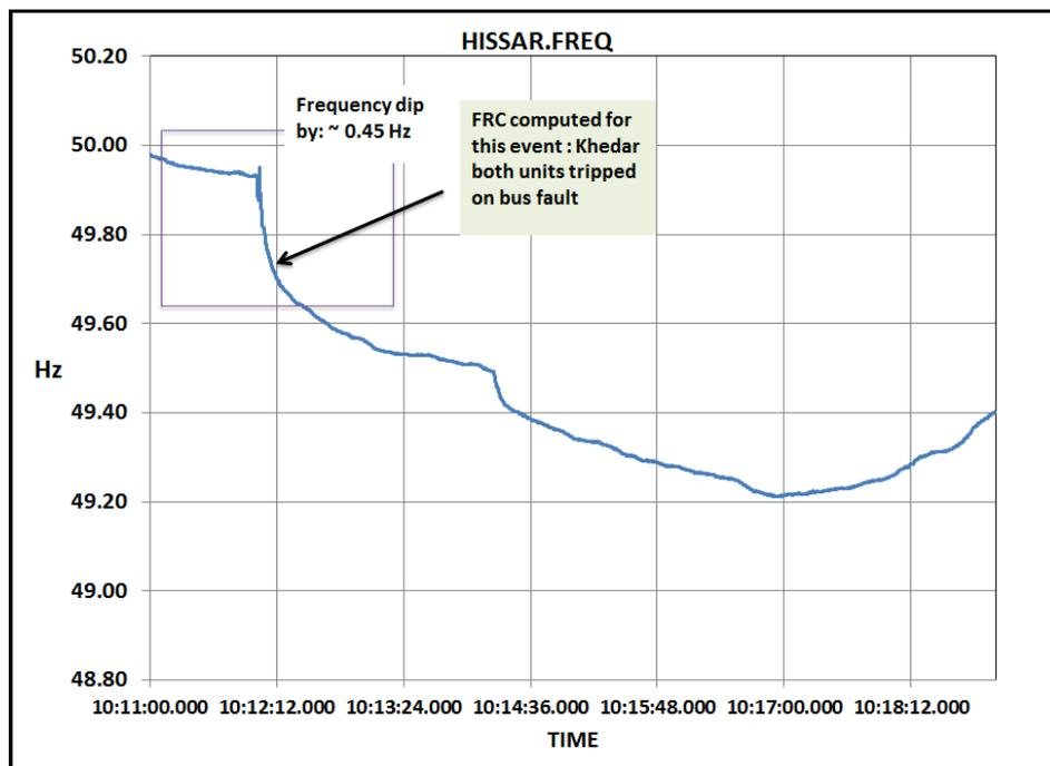
Figure 130: Hissar frequency during generation loss of 1100MW at Khedar TPS in Haryana
